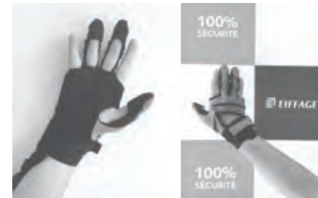
"Bionic" glove developed in partnership with Bioservo Technologies AB © Eiffage Infrastructure division
